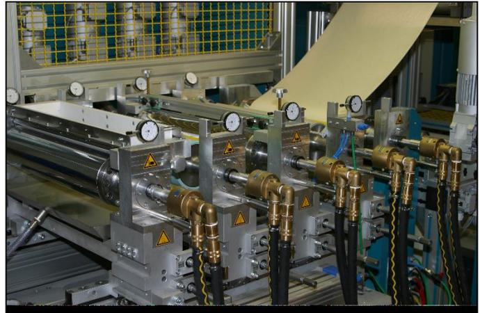
The application of hotmelt adhesives is another possibility with the new demonstration line. The melted adhesive is continuously pumped to the heated slot die.
