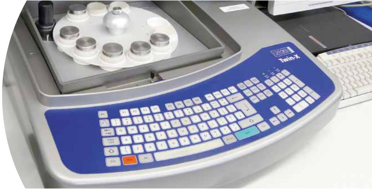
X-ray tester to determine silicone coat weights.
