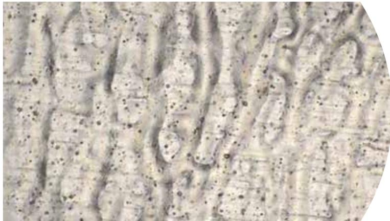
Silicone coating with worn application roller
