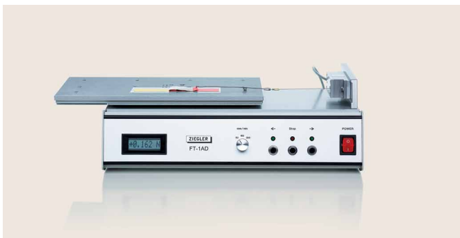
PICTURE 4: Peel adhesion (FINAT test method 1 & 2)
